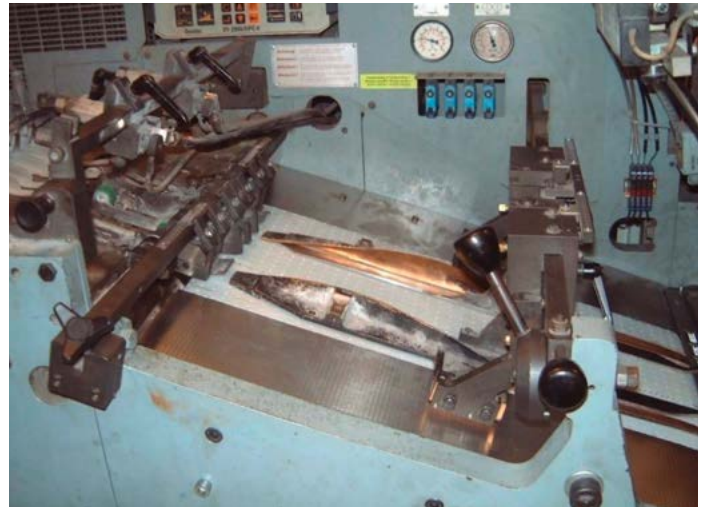
Side flap folding section with vacuum belt transport
