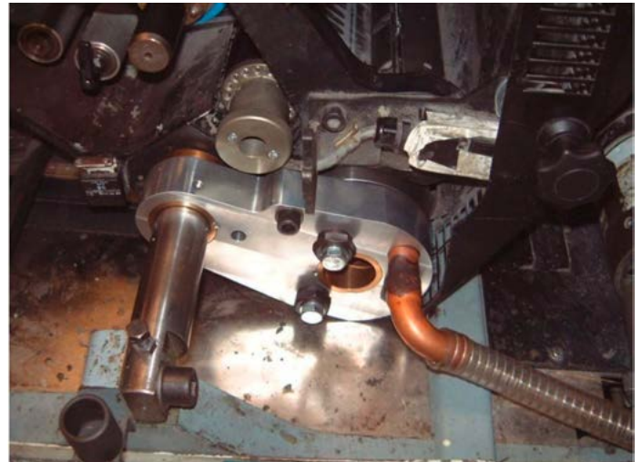
Second control valve on the window material conveying cylinder
