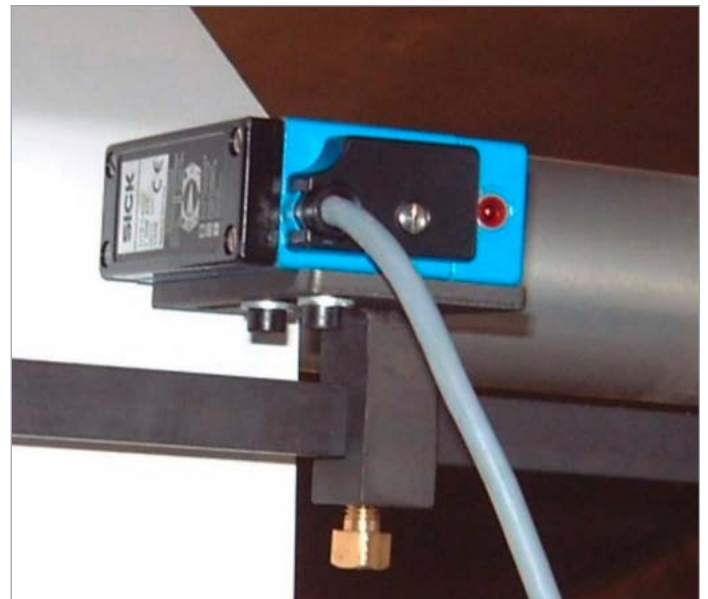
Mark reader to detect printed registration mark
