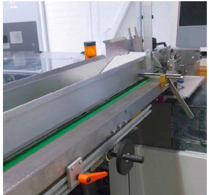
Size changes require the fast and precise adjustment of the conveyor belt at the envelope feeder to ensure a smooth and interruption-free running of the machine at maximum production speeds.
