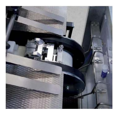
The gripper guides of the proven W+D BB700 14K are more rigid than those of the newer 16K models. This leads to increased wear and tear on the grippers and the guide bars and to an unreliable or nonparallel envelope transport.
