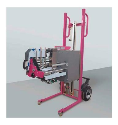
W+D inserting systems are particularly variable due to their modular design. That makes it possible to move feeders within the machine. But they can also be used in different machines. Since the weight of the feeders varies between 20 kg and 60 kg, depending on the type, exchanging them can also be a real feat.
