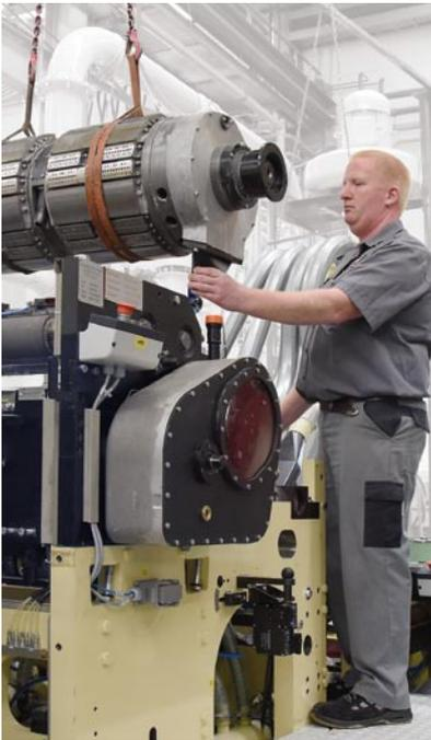
Exchanging the folding cylinder in a W+D 624.03
